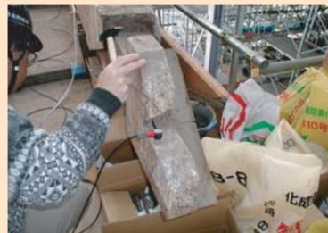
Stress wave measurement for nondestructive inspection.
